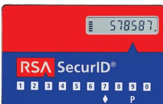
The RSA SecurID 520 PINpad model is the same size as the RSA SecurID 200 but has a PINpad feature that enables users to encrypt their passcode for a higher level of security.
