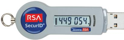
The RSA SecurID 800 offers the one-time password functionality of the other hardware authenticators and can be used for storage of Windows® username/password credentials and digital certificates—creating a master key for multiple authentication methods. When connected, the RSA SecurID 800 is enabled for automatic token code entry, allowing applications to programmatically access token codes directly off the device and eliminating the need for the user to type their code.
